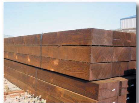
Douglas Fir Bridge Stringers
