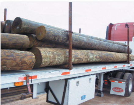
Southern Yellow Pine Piling
